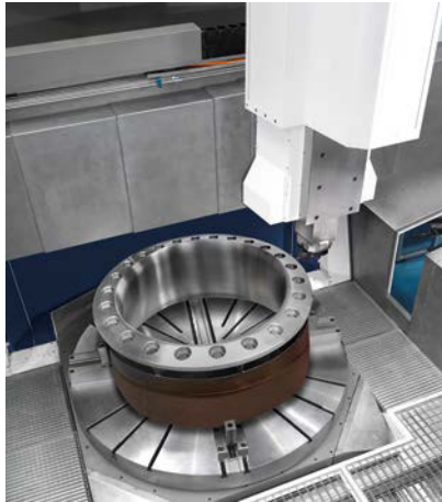
▲ Engine casing turning / drilling
